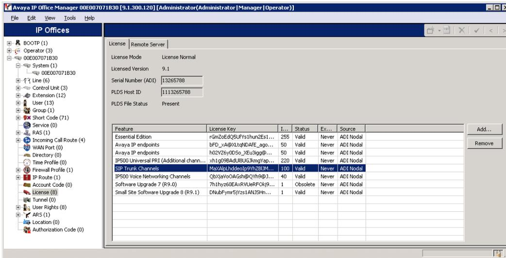
The screenshot shows the 'Avaya IP Office Manager' application window. The 'License' tab is active, displaying the 'Remote Server' configuration. The 'License Mode' is set to 'License Normal', and the 'Licensed Version' is '9.1'. The 'Serial Number (ADI)' is '13265788' and the 'PLDS Host ID' is '1113265788'. Below this, a table lists various licenses:
